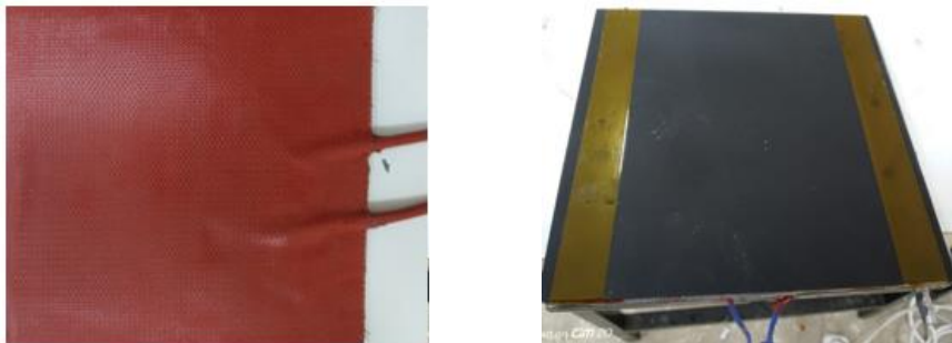
Fig. 3 20V Silicon heater and a mimic of battery cell
