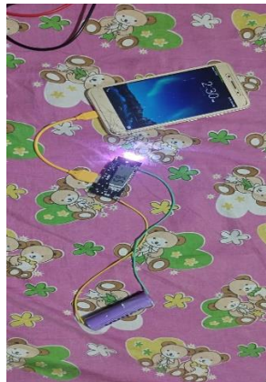
Fig. 16 Mobile charging using stored harvested rechargeable battery
