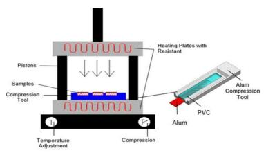
Fig. 2 Schematic representative of hot press equipment
