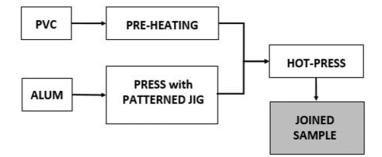
Fig. 1 A schematic picture of the sample preparation process
