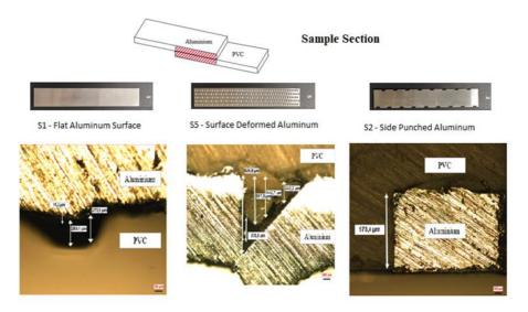
Fig. 6 Optical microscope result of interface on S1, S5 and S2
