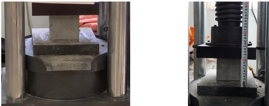
Fig. 8. Compression test of concrete cube
