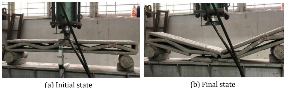
Fig. 9. The failure mode of CB00
