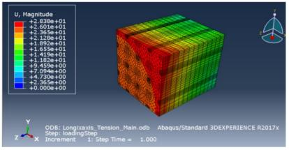
Fig. 7. Resultant displacement on implementation of longitudinal stress
