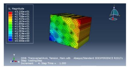
Fig. 5. Resultant displacement on implementation of transverse stress
