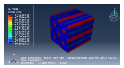
Fig. 6. Postprocessing of longitudinal modulus
