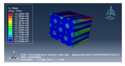
Fig. 4. Postprocessing of transverse modulus
