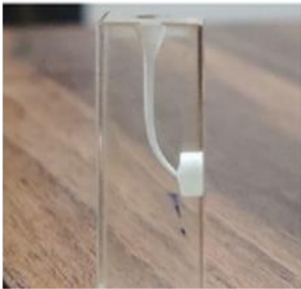
Fig. 2. Endo training block prepared with uniform 6% taper under scope of study (17)
