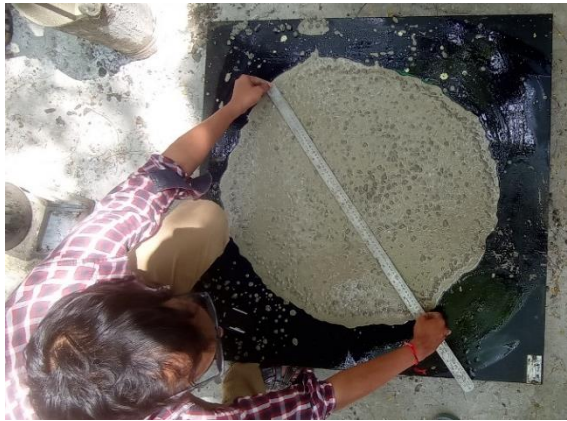
Fig. 4. Slump flow of DC0 mix proportion
