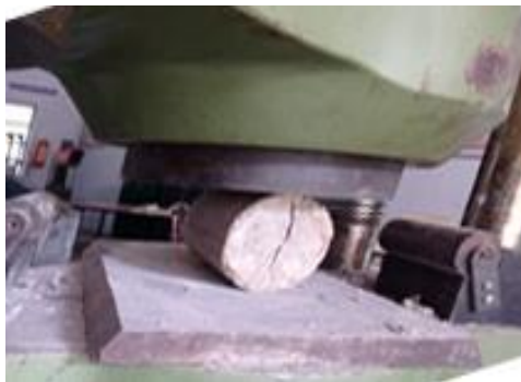
Fig. 2. Split tensile test on SCC specimen
