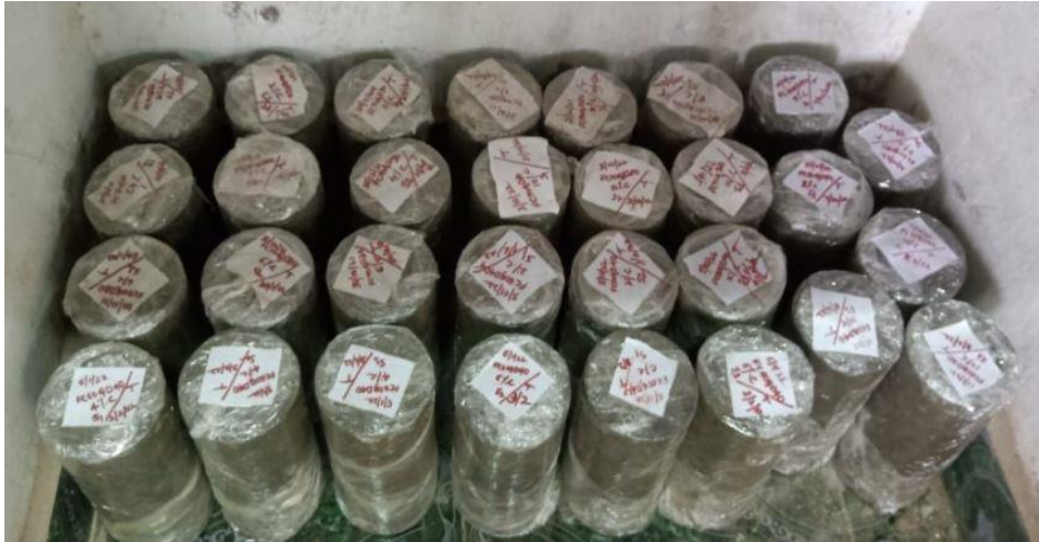
Fig.3 Cylindrical test specimens wrapped in polyethylene sheet
