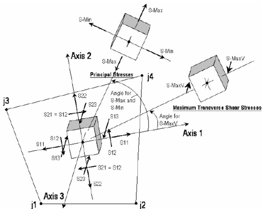
Figure 14. Internal stresses in shell element [20]
