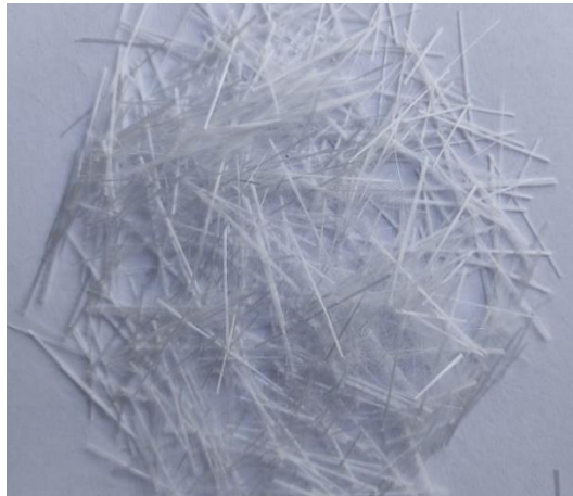
Fig. 3 E-glass fiber Chopped roving of length 1" (inch)
