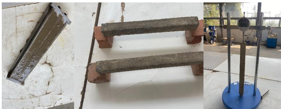
Fig. 5 Drying shrinkage test using length comparator
