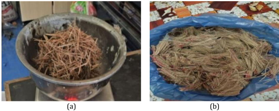
Fig. 3 Micro Reinforcement Bamboo (a) and Hemp (b)
