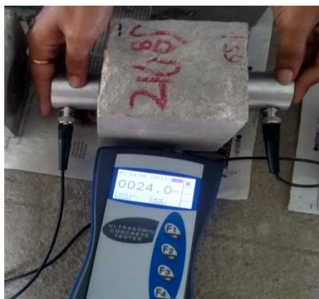
Fig.4 Setup of UPV measurement
