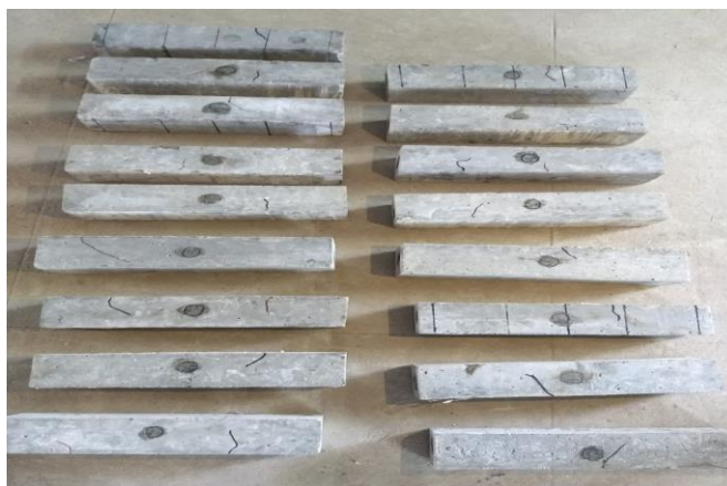
Fig. 2. Setup of cracked concrete specimens
