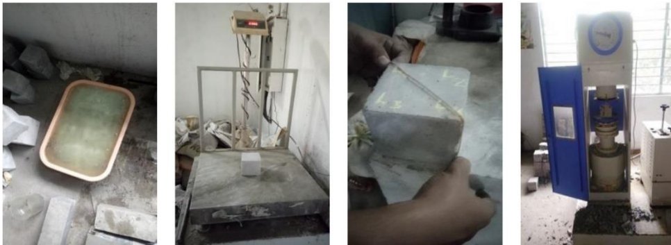
Fig. 3 Experimental setup for acid attack test
