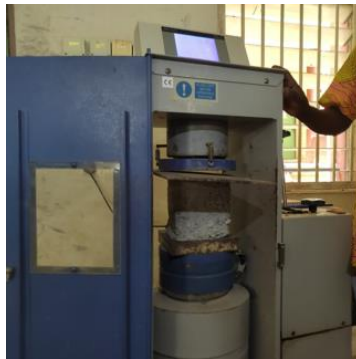
Fig. 3 Compressive strength test
