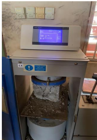
Fig. 9 Failure mode of glass waste in concrete
