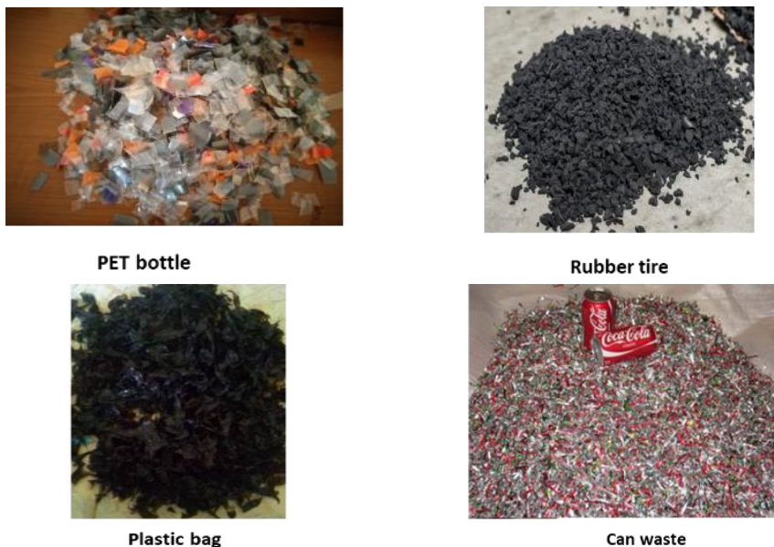
Fig. 2 Waste materials used for partial replacement of natural aggregate
