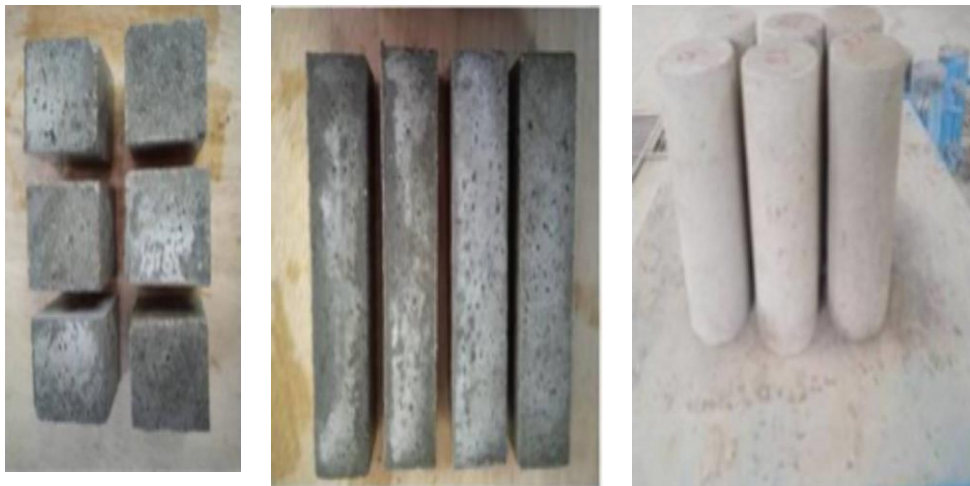
Fig. 4 Cast samples to physical and mechanical properties
