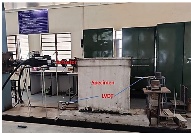
Fig. 8 Experimental setup of the raft and wall connection
