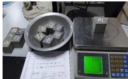
(h) Water absorption test
