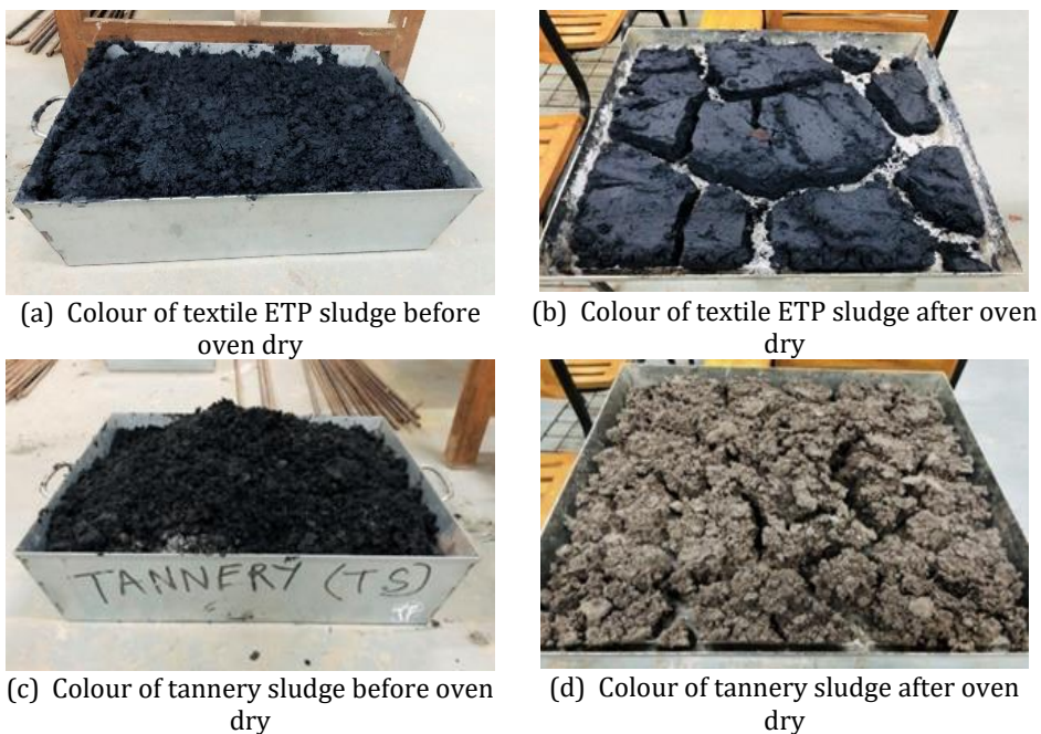
Fig. 2 Colour of textile ETP and tannery sample before and after the oven dry process
