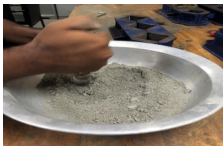
Fig. 3 Hammering of oven dry sludge to make it powder
