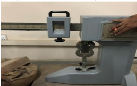
(g) Tensile strength test of mortar
