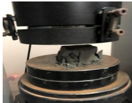
(f) Compressive strength test of mortar
