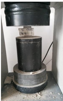
Fig. 8 Compressive test showing the crushing of specimen.
