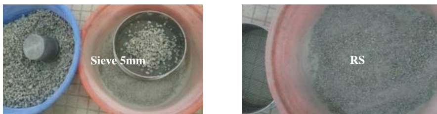
Fig. 1 Preparation of recycled sand by sieving
