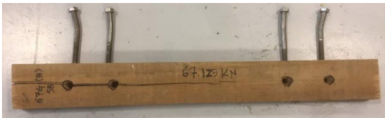
(b) Group 7 with e_t = 125 mm and s_b = 100 mm
