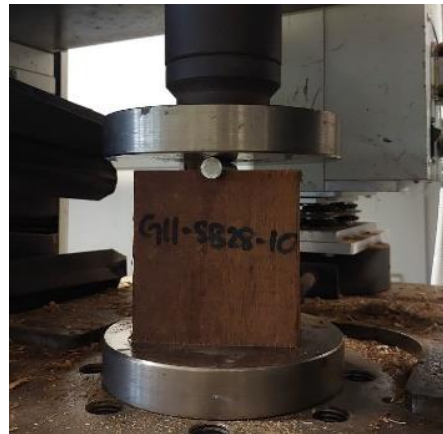
Fig. 4 Embedding strength test setup
