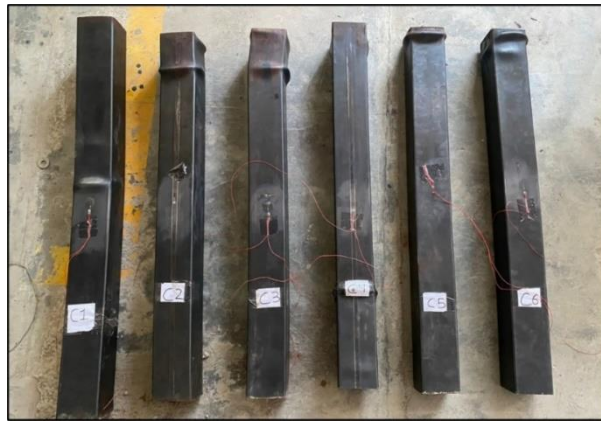
Fig. 4. Failure mode in experimental investigation
