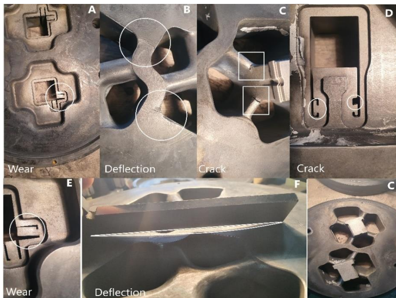
Fig. 2. The most important failures of aluminum extrusion dies
