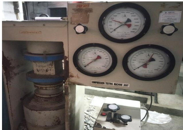
Fig. 4. Compressive strength test using 300T CTM
