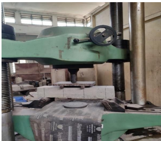
Fig. 8. Flexural strength test using 100T UTM
