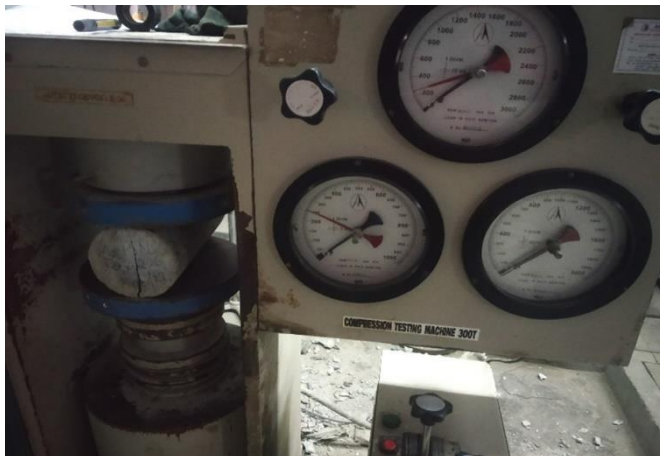
Fig. 6. Split tensile strength test using 300T CTM
