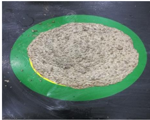
Fig. 2. Slump flow diameter of fresh SCC
