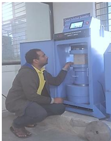
Fig. 3. Compressive strength testing machine apparatus
