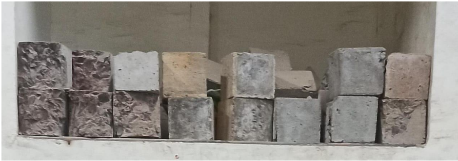
Fig. 4. SCC specimens after compressive strength testing
