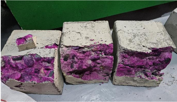
Fig. 11. Concrete samples after phenolphthalein test
