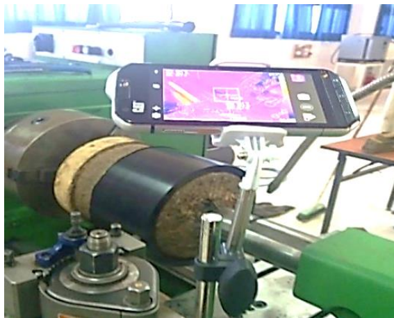
Fig. 2. Temperature measurement set-up using CAT S60 smartphone [13]
