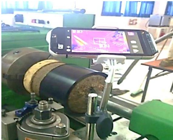
Fig. 2. Temperature measurement set-up using CAT S60 smartphone [13]
