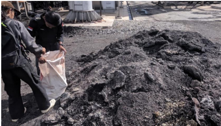
Fig. 3. Slag from burning palm shell ash
