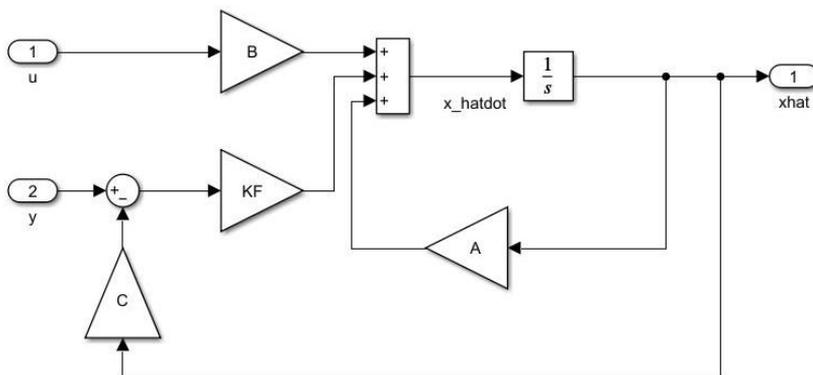
Fig. 7. The structure of the Kalman filter
