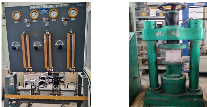
Fig. 5. Concrete permeability test setup
