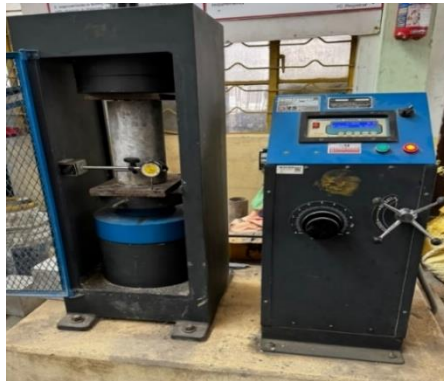
Fig. 3. Setup for stress- strain behavior
