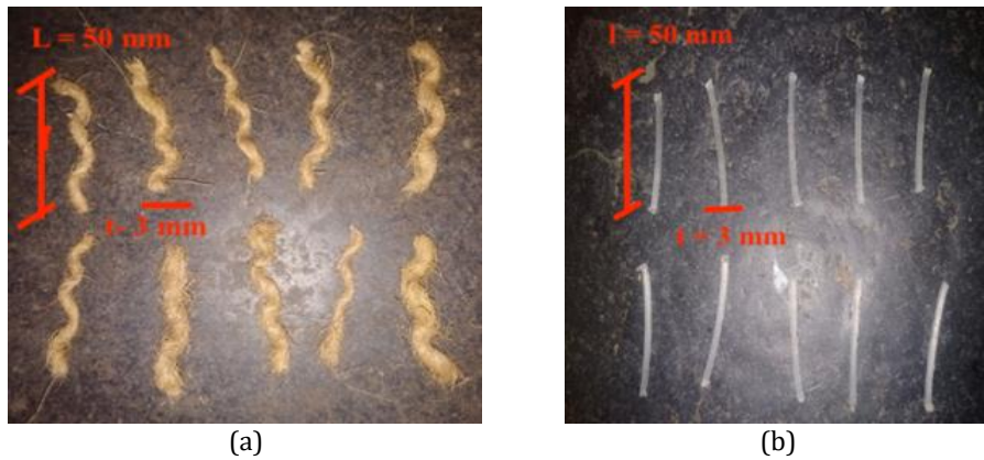
Fig. 1. (a) Coir fiber (b) plastic fiber
