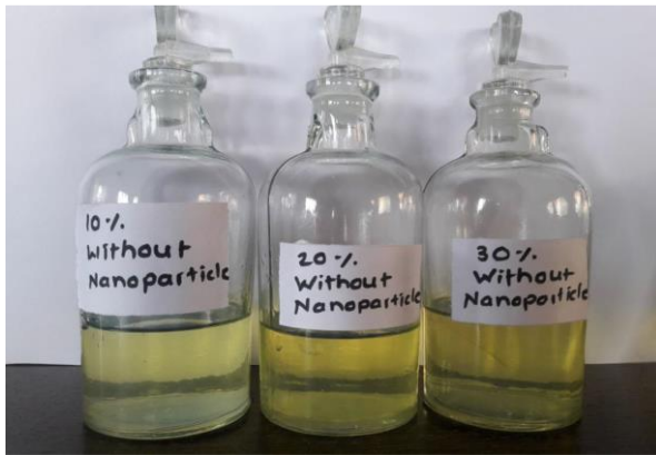
Fig. 3. Samples of Diesel blends with Simarouba glauca Methyl Ester (B10, B20, B30) [19]
