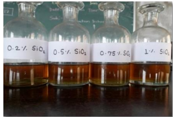
Fig. 4. Simarouba glauca Methyl Ester with SiO 2 nanoparticles samples prepared for experimentation [19]
