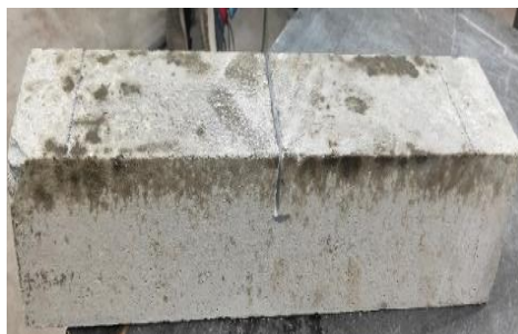
Fig. 6. Notched beam sample
