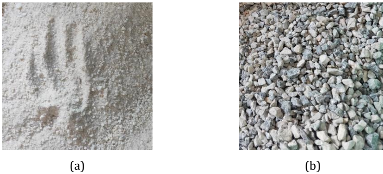
Fig. 2. (a) Fine aggregate (stone dust) and (b) Coarse aggregate (granite)
