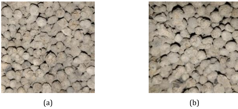
Fig. 3. (a) Sintered fly ash lightweight aggregate, Fraction: 4-8 mm and (b) Sintered fly ash lightweight aggregate, fraction: 8-16 mm
