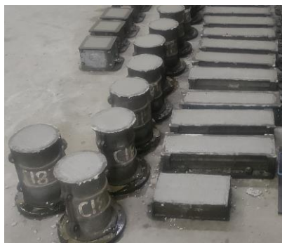
Fig. 5 Concrete cubes, cylinders, and beams in molds
