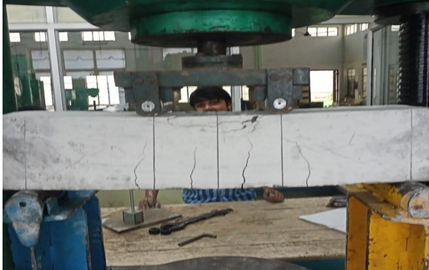
Fig. 9. Specimen crack for 70% reinforcement
