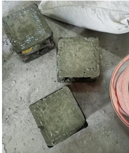
Fig. 3. Wet concrete cubes after casting
