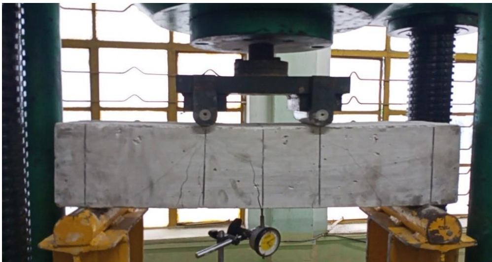
Fig. 8. Specimen crack for 100% reinforcement
