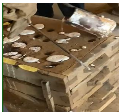
Fig. 4. Sand mould with the composites
