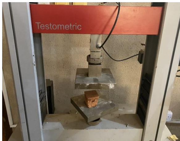
Fig. 8. Image of a failed Refractory Bricks under cold crushing strength test
