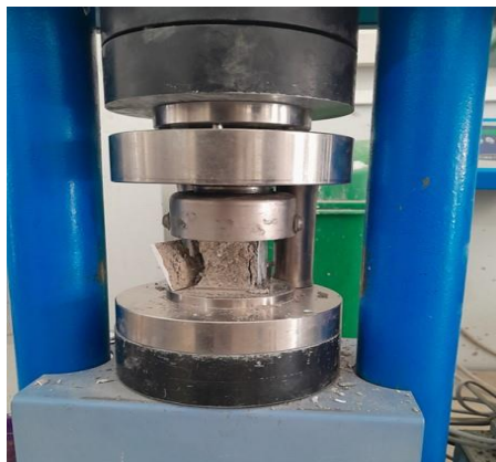
Fig. 5. Compressive strength test of geopolymer mortar
