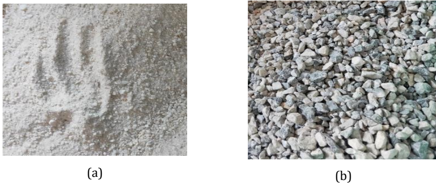
Fig. 1. (a) Fine aggregate (crushed) and (b) coarse aggregate (granite)
