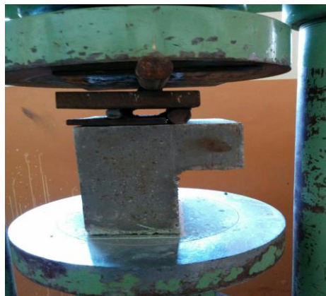
Fig. 9. Details of the shear test
