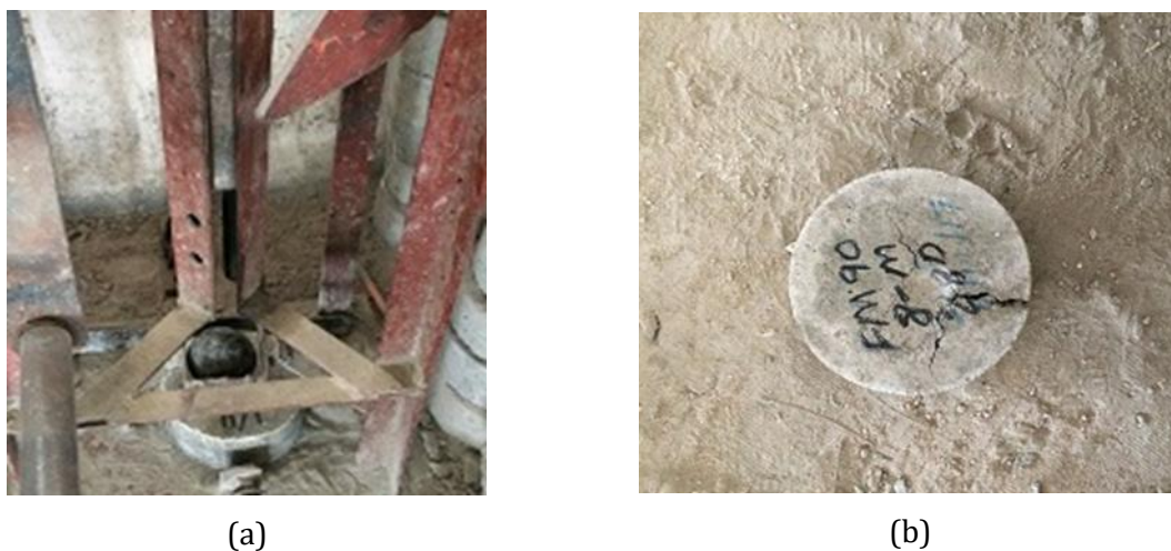
Fig 11. (a) Impact test setup; (b) failure of impact specimen
