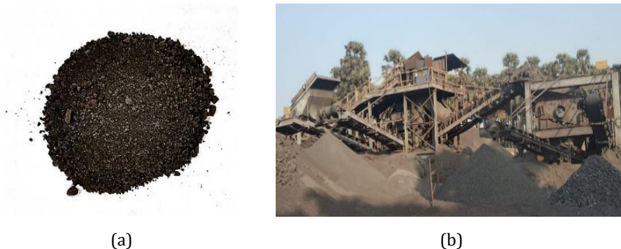
Fig. 3. (a) Electric Arc Furnace (EAF) Slag Fine Aggregates and (b) processing of Electric Arc Furnace (EAF) steel slag
