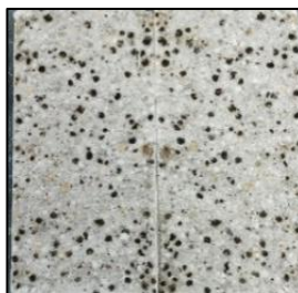
Fig.12. Fractured lightweight concrete specimen after split tensile test
