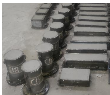
Fig. 6. Concrete cubes, cylinders, and beams in molds
