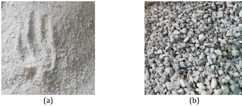
Fig. 1. (a) Fine aggregate (stone dust) and (b) Coarse aggregate (granite)
