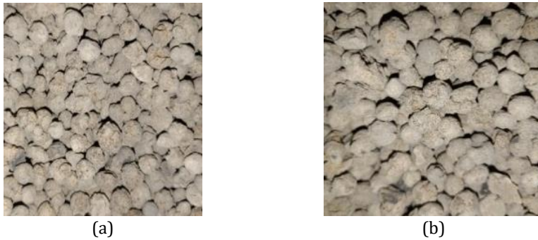
Fig.2 . (a) Sintered fly ash lightweight aggregate, Fraction: 4-8 mm and (b) Sintered fly ash lightweight aggregate, fraction: 8-16 mm
