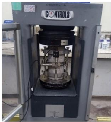
Fig. 8. Test setup for stress strain behavior and modulus of elasticity of concrete of concrete
