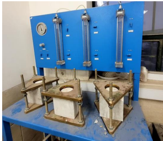
Fig. 11. Concrete permeability device
