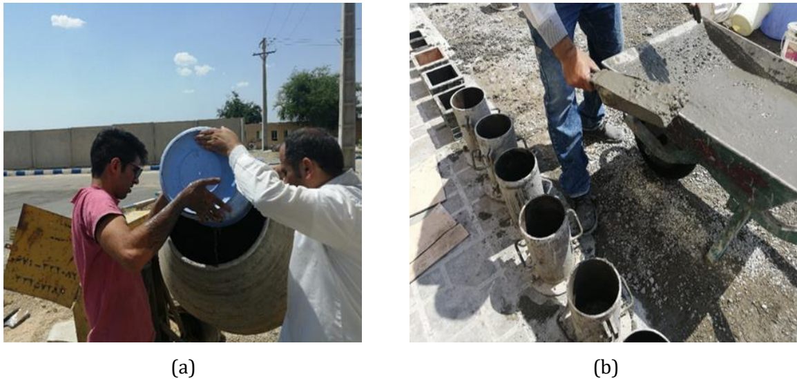
Fig 3. (a) Adding water, bentonite and carbon to concrete and (b) molding samples with concrete
