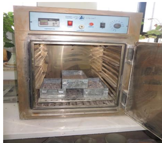
Fig. 2. A sample of sand in order to measure the moisture content of the materials
