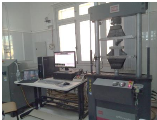
Fig. 8. The ASTM C192 testing set-up
