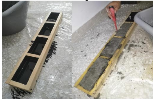
Fig. 4. The specimen's concrete pouring
