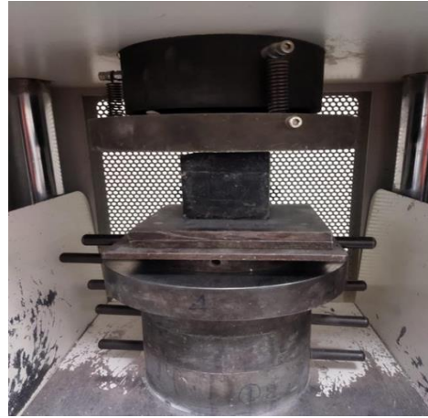
Fig. 6. Compressive Strength Test
