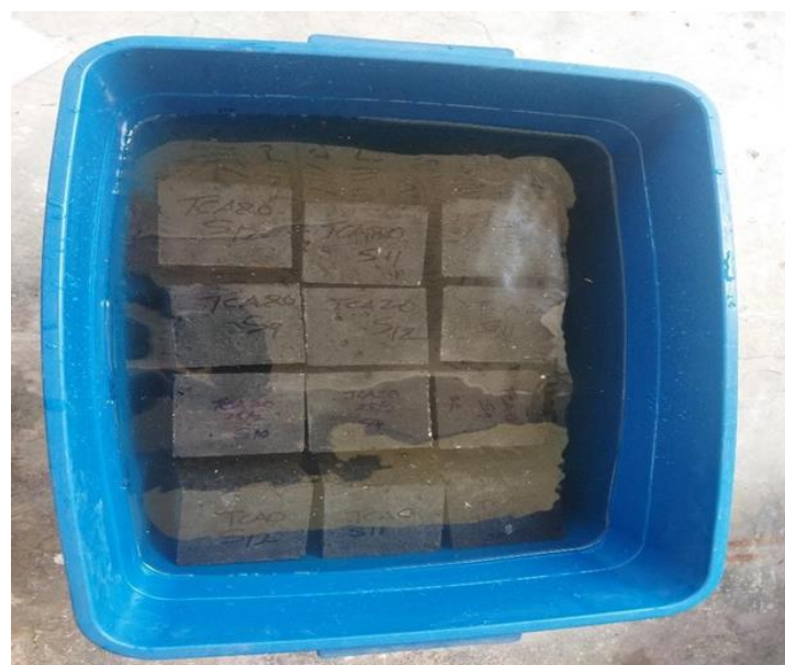
Fig. 12. Sulphate Resistance Test
