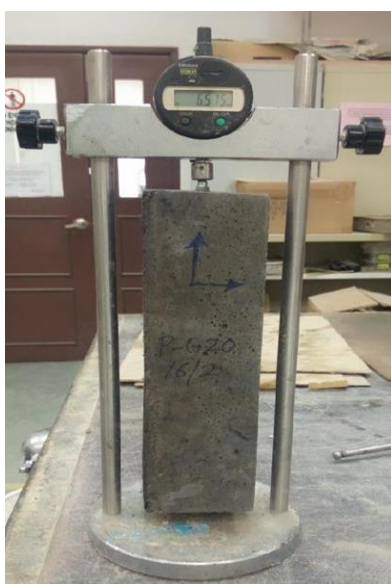
Fig. 11. Drying Shrinkage Test
