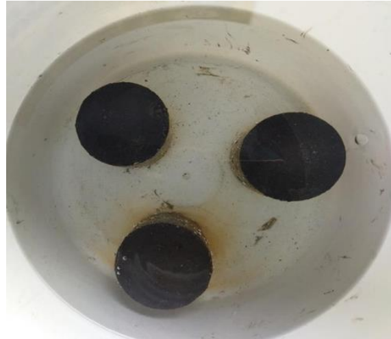
Fig. 10. Water Absorption Test
