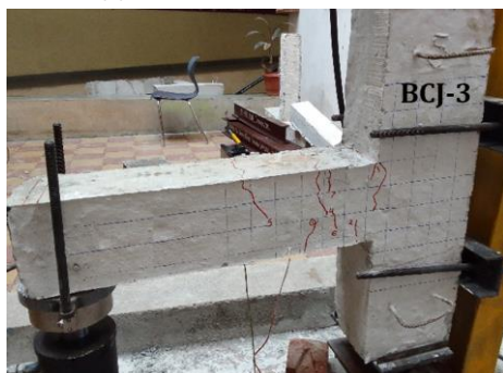
(a) Crack Patterns of BCJ-3
