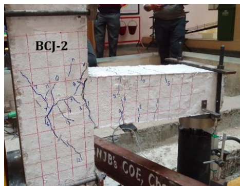
(a) Crack Patterns of BCJ-2
