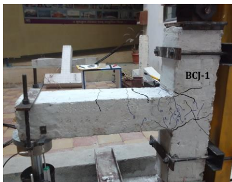
(a) Crack Patterns of BCJ-1
