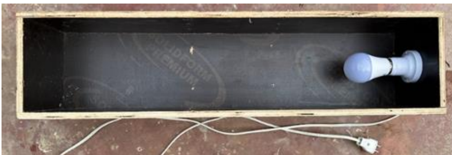
Fig. 8. Light transmissibility test setup without the sample, cover, and lux meter
