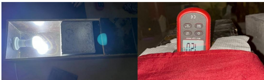
Fig. 9. Light transmissibility test setup without the sample, cover, and lux meter
