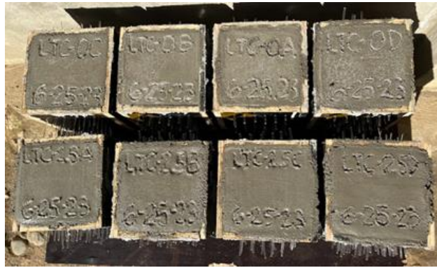
Fig. 5. Samples casted on the molds
