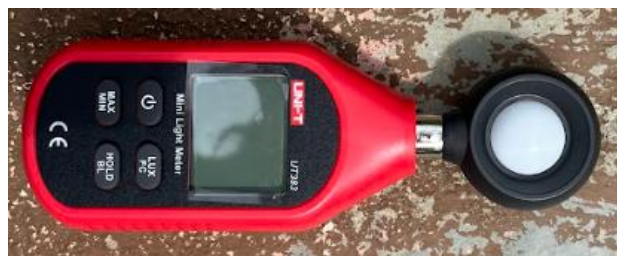
Fig. 6. Lux meter used for the Light Transmissibility Test
