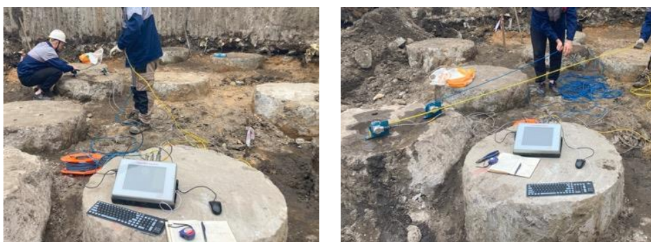
Fig. 6. Field photographs of the CSL testing procedure for bored piles
