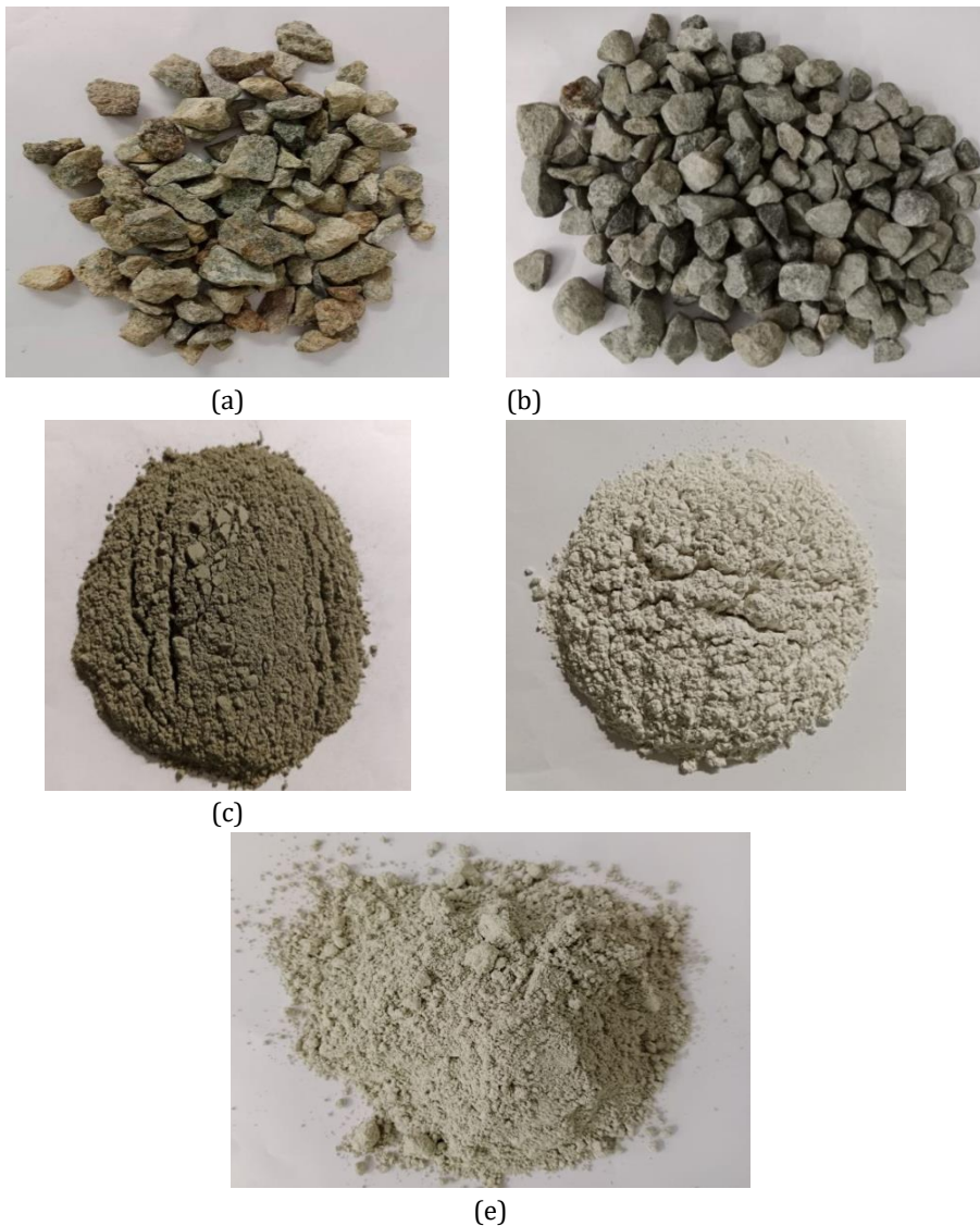
Fig. 2. Images of the materials used in the current study (a) recycled aggregate, (b) natural aggregate, (c) cement, (d) ggbs and (e) I – crete
