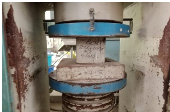
Fig. 5. Compressive strength test
