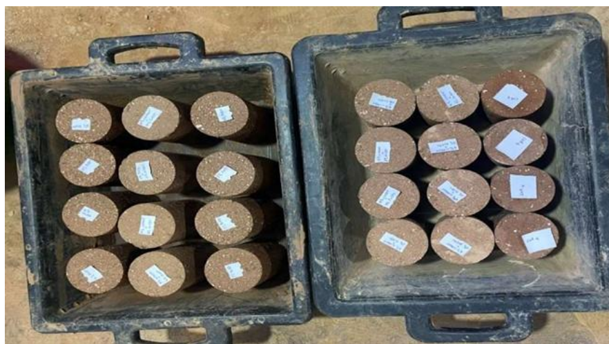
Fig. 8. CEB samples tested during compressive strength tests
