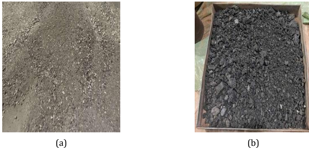
Fig. 2. (a) Soil from Casablanca; (b) Natural pozzolana
