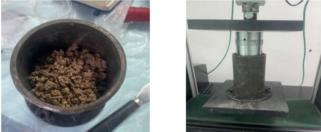
Fig. 4. Experimental set-up of the compaction tests
