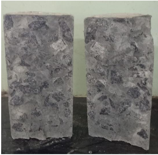
Fig. 12. Damaged NMA 100% RA cylinder
