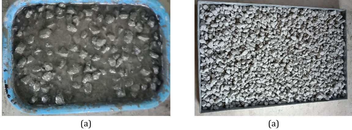
Fig.4. (a) RA soaked in cement slurry and (b) Surface-dried RA (Treated Aggregates)
