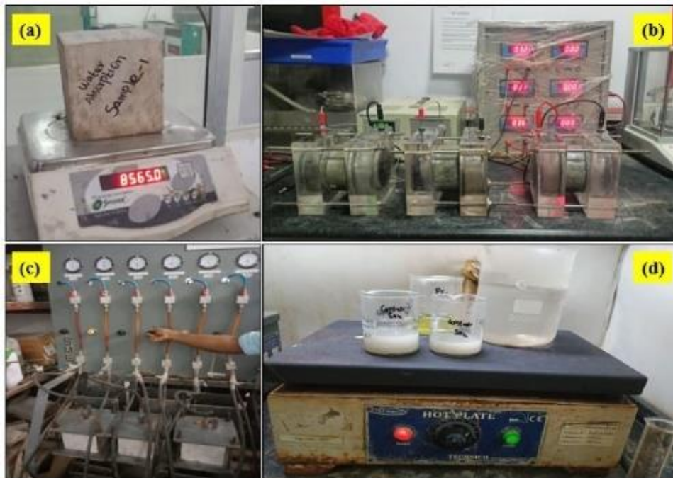
Fig. 1. Effect Experimental test setup: (a) Water absorption test, (b) Rapid chloride penetration test, (c) Water penetration test, and (d) Acid and sulphate solution preparation
